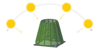
The core of the GICON® photobioreactor is the flexible silicone-based tubing system as a result of the successful cooperation between GICON® and Wacker Chemie AG. The highly transparent ELASTOSIL® silicone rubber and innovative double wall system provide a very convincing a solution for indoor and outdoor use.
